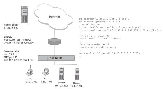
Figure 6 shows an example of a network using dynamic NAI on a ServerIron ADX ADX. The device is acting as a gateway to connect a private network to the Internet. The private network, which can also be considered as the **inside** network, is using IP addresses in the range of 10.10.1.2 - 10.10.1.254 with a 24-bit subnet mask.
